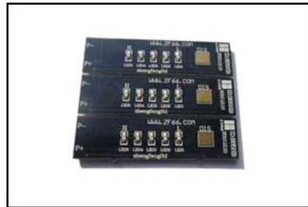
Name: LED Indicator for 16 Cells Battery Model No.: ZFB55HB Size: 60.1 × 15.6 × 3.6mm
