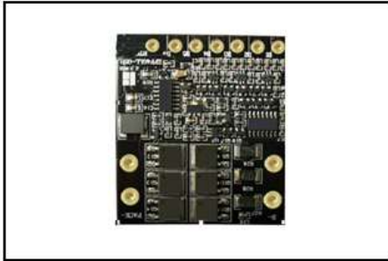
Name: PCM for 5 Cells Lithium Battery Model No.: ZFE20LL-05A Size: 56.5 × 51 × 4mm
