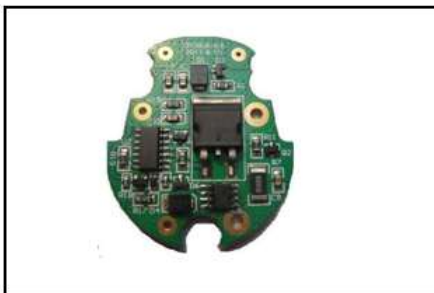
Name: PCM for 10.8V Dynamic Battery Model No.: ZFC10LR-11E Size: 38 × 44.5 × 7.5mm
