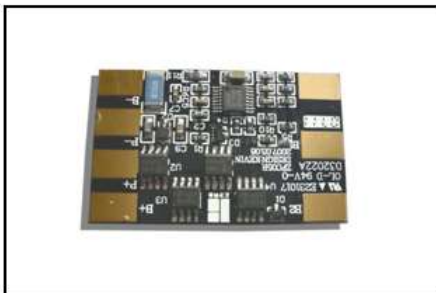
Name: PCM for 10.8V Lithium Battery Model No.: ZFC10LR-03A Size: 28 × 46 × 2.7mm
