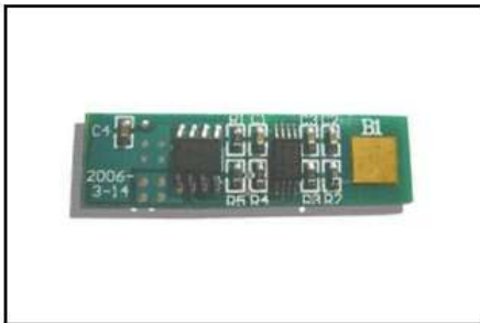
Name: PCM for 7.4V Li Battery Model No.: ZFB03LR-05 Size: 35 × 10 × 2.7mm
