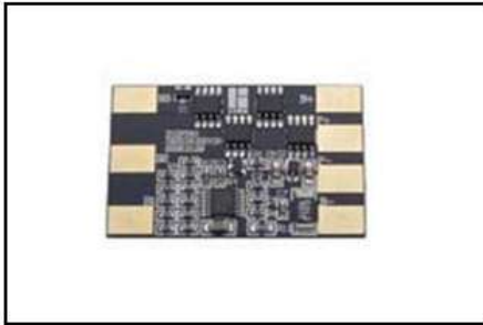
Name: PCM for 14.4V Lithium Battery Model No.: ZFD10LR-03A Size: 28 × 46 × 2.7mm
